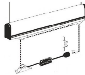
Double pulley bottom rail Constant tension spring. Ideal for sloping windows.
